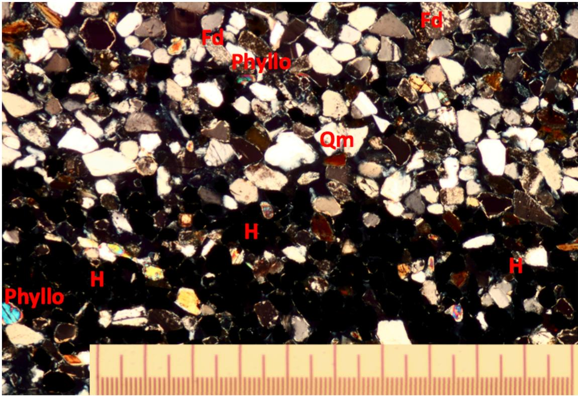
Sample LBF\_FWSED1 under cross-polarized light and 16x magnification. Horizontal lamination of opaque minerals identified as magnetite. Oriented so that the photomicrograph is perpendicular to bedding and top is up-section. Scale bar is 1mm.
