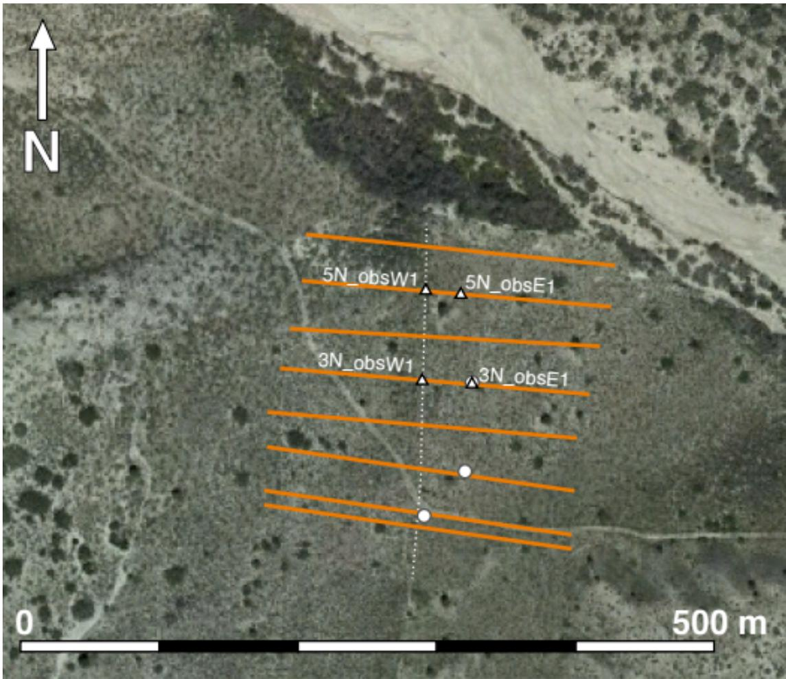
**Figure 6** – Satellite imagery of the north end of the Loma Blanca fault. The dotted line represents the fault, orange lines represent geophysical resistivity transects perpendicular to the fault, circles represent location of directional boreholes drilled west to intersect the fault with core recovery, and triangles represent location of monitoring wells.
