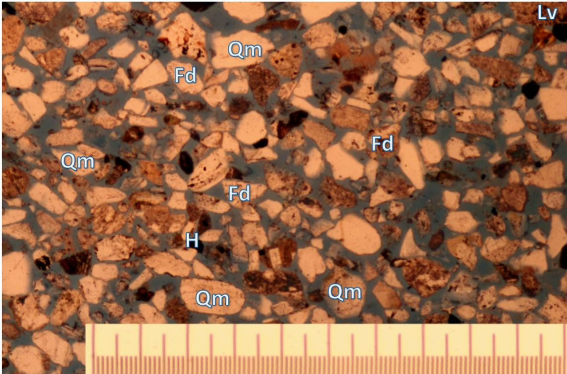
**Figure 4** - Polarized photomicrograph of sample LBF\_FWSED2 with 16x magnification. The sample is perpendicular to weak bedding observed in outcrop and is oriented with up being the top of the photo. The sand is compositionally similar to LBF\_FWSED1 with differences in heavy mineral distribution. LBF\_FWSED2 also exhibits slightly more intergranular pore space indicated by blue epoxy. Scale bar is 1mm.
