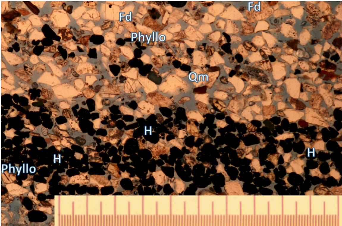
**Figure 3** - Polarized photomicrograph of sample LBF\_FWSED1 with 16x magnification. The sample is perpendicular to bedding and is oriented with up being the top of the photo. Monocrystalline quartz grains are angular to sub-angular with the addition of intact, unaltered feldspars and phyllosilicates indicating an immature sand. Sample shows no noticeable cementation in intergranular pore space. Scale bar is 1mm.
