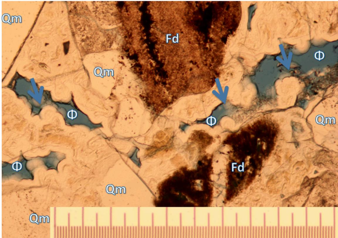
**Figure 2** - Polarized photomicrograph of sample LBF\_0212\_1B with 16x magnification. With further magnification, the opal cement is more defined and seen nucleating from framework grains filling intergranular porosity. Scale bar is 1mm.
