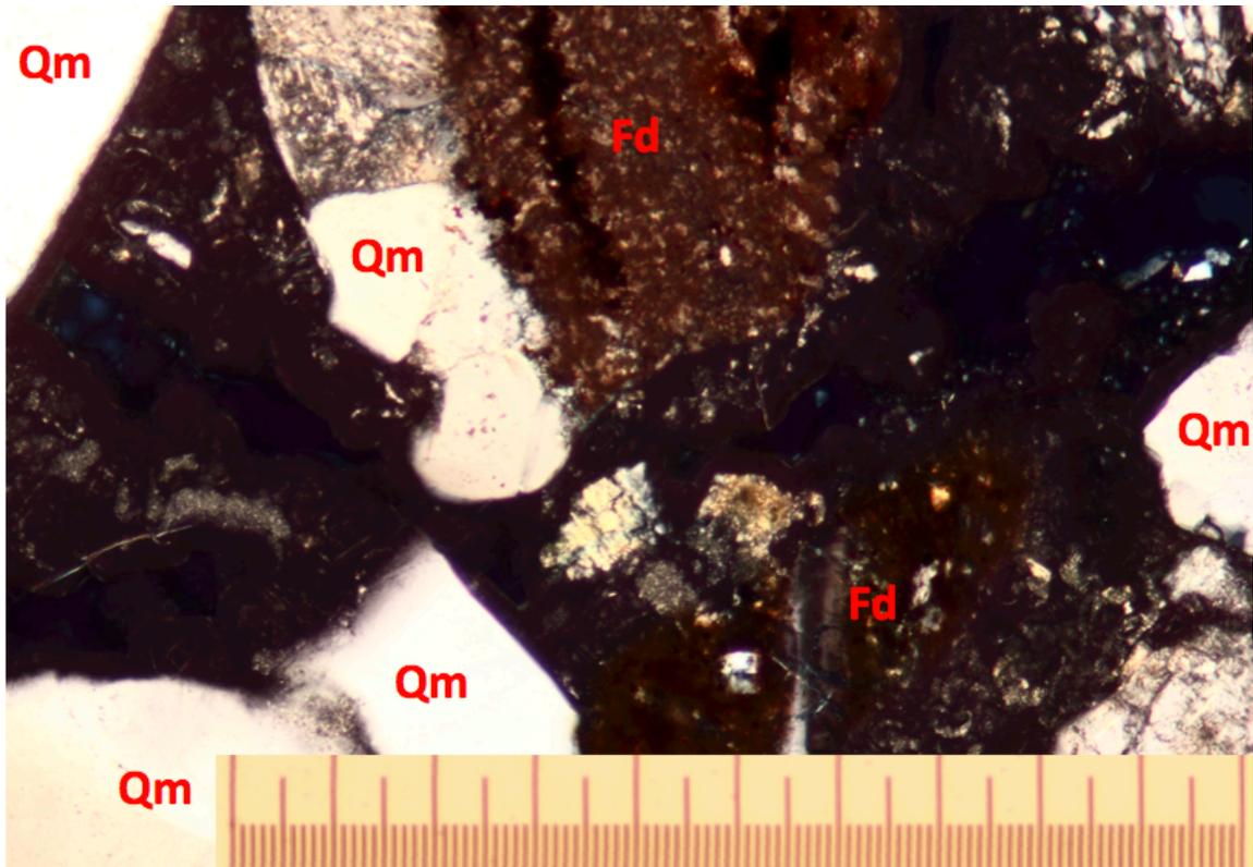
Sample LBF\_0212\_1B under cross-polarized light and 16x magnification. Opal appears opaque/black in the image. Scale bar is 1mm.
