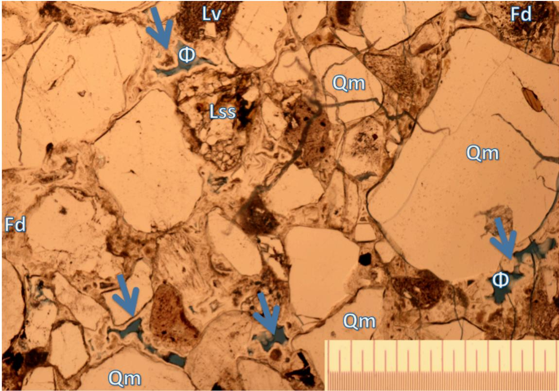
**Figure 1** – Polarized photomicrograph of sample LBF\_0212\_1A with 8x magnification. The sample is composed of monocrystalline quartz (QM), feldspars that show levels of sericite alteration (Fd), lithic volcanic fragments (Lv), and lithic sedimentary fragments (Lss). The  $\phi$  symbol over blue epoxy indicates areas of intergranular porosity. Blue arrows highlight botryoidal opal cementation. Scale bar is 1mm.
