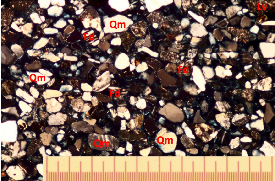
Sample LBF\_FWSED2 under cross-polarized light and 16x magnification. Oriented so that the photomicrograph is perpendicular to bedding and top is up-section. Scale bar is 1mm.
