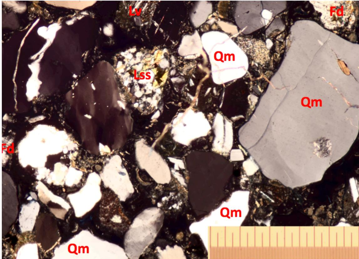
Sample LBF\_0212\_1A under cross-polarized light and 8x magnification. Opal appears opaque/black in the image. Scale bar is 1mm.
