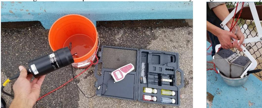
Figure 4: Uvilux Tryptophan fluorometer used in surface water samples (left) and sediment dredge and washbowl for collecting bottom sediments (right)
