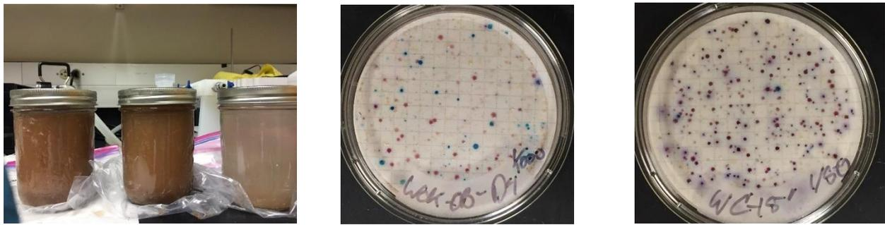
Figure 2: Sediment and surface water microcosms (left) and incubated MF plate bacteriological results (right)
