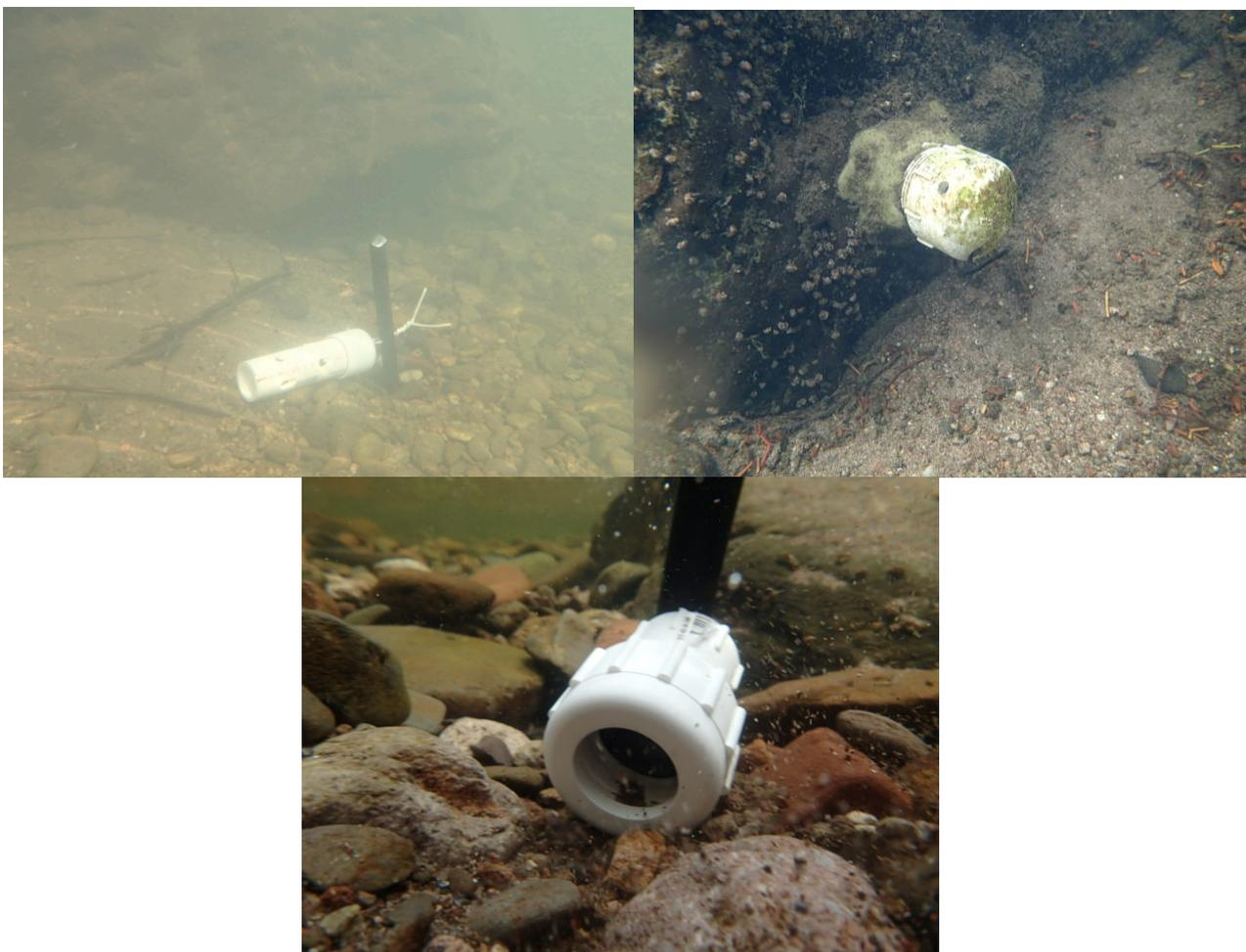
**Figure 1:** Types of temperature loggers used include ProV2 (top left), Tidbit v2 (top right), and the adapted Stream Temperature, Intermittency, and Conductivity (STIC) logger (bottom). ProV2 and STIC models are anchored with three foot framing stake and ten gauge wire, Tidbit v2 model is affixed to a permanent stream structure using two-part waterproof epoxy.
