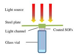
Figure 1. Batch photoreactor with catalyst-coated SOFs
