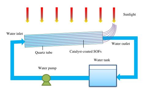
Figure 2. Continuous-flow photoreactor with catalyst-coated SOFs
