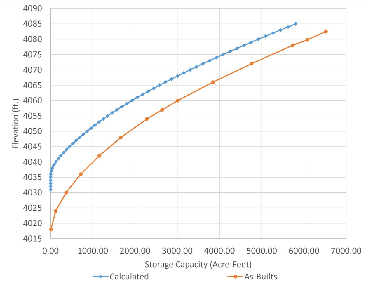
Figure 8: Stage Storage Capacity
