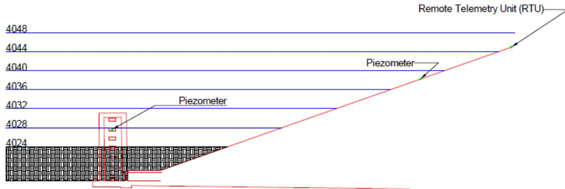
Figure 11: Proposed piezometer placement on ABM1
