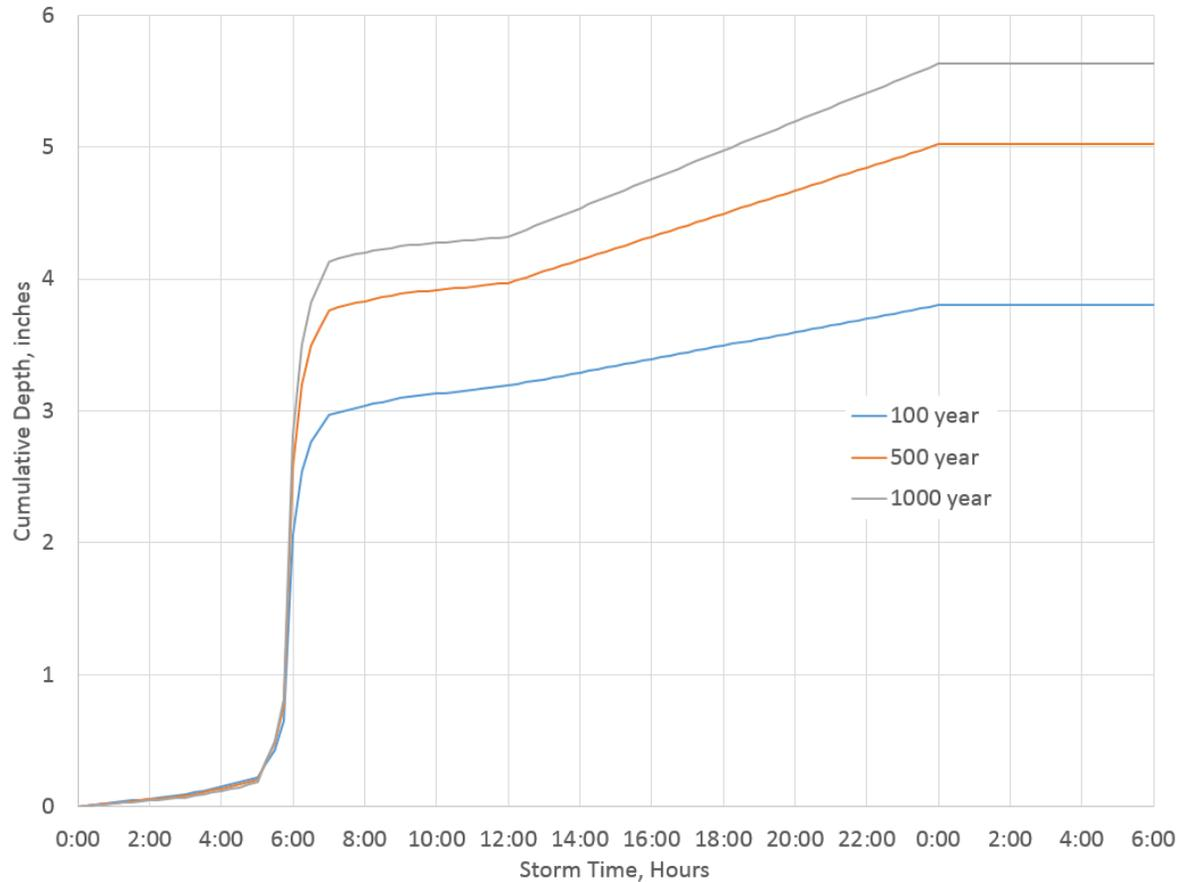
Figure 7: NRCS Type II-75 Hyetograph
