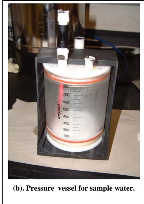
(b). Pressure vessel for sample water.
