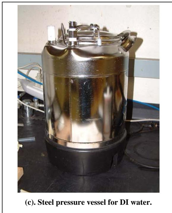
(c). Steel pressure vessel for DI water.
