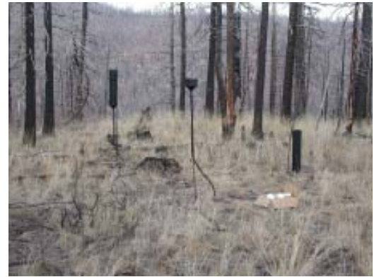
Precipitation collectors at a site outside Los Alamos, New Mexico. The different collector designs allow determination of the isotope signatures of fresh snow and infiltration water derived from snowmelt.
