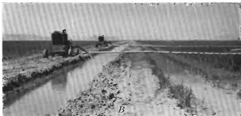
B. WATER FROM STRIBLING WELL BEING DISTRIBUTED THROUGH SPRINKLER SYSTEM BY PORTABLE DIESEL-POWERED CENTRIFUGAL PUMPS.
