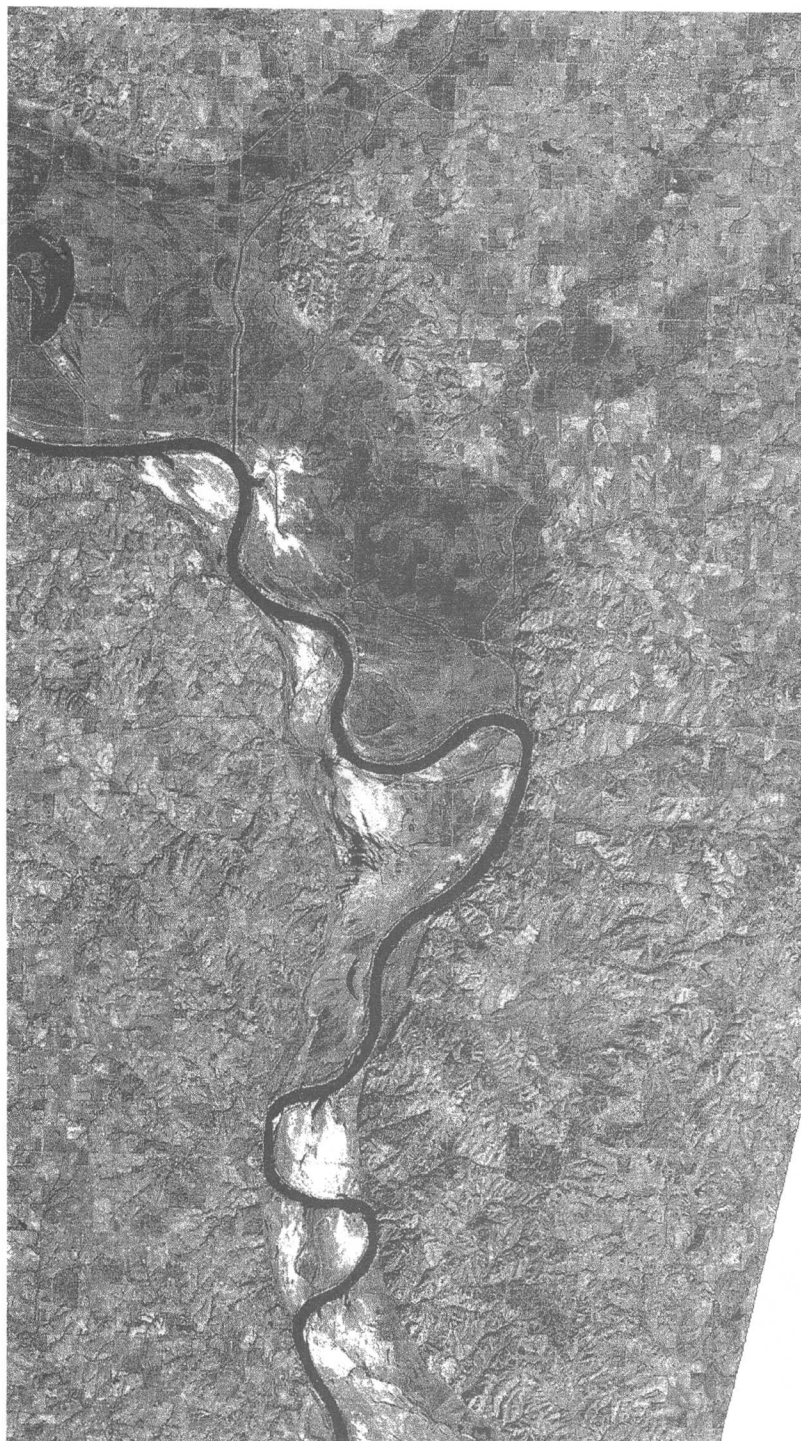
Landsat Thematic Mapper satellite image showing post-1993 flood conditions near Glasgow, Mo. River flow at this time was approximately 8 percent of the flow during peak flood conditions. Nine large levee failures occurred in the area of this scene during the 1993 floods. Associated areas of thick to moderately thick sand deposits (generally greater than 15 centimeters thick) are shown as white areas on this image. Date of acquisition December 7, 1993.
