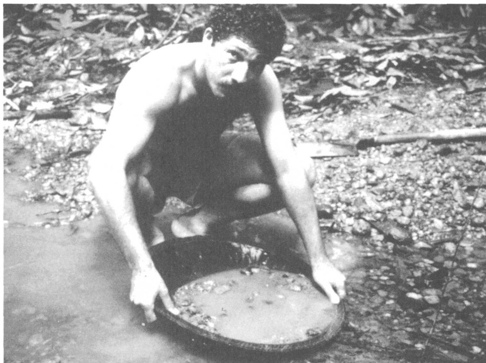
Figure 2. Gold miner panning ore using a wooden "batea." Mercury is added to the panned concentrate and combines with minute gold particles to form an amalgam. The amalgam is then "roasted" (commonly by using a blowtorch), and mercury is driven off as a vapor. Unused liquid mercury is often lost to the river.
