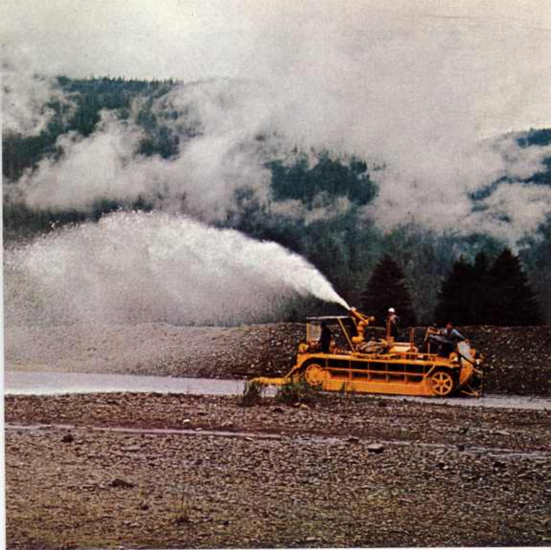
Riffle sifter in Alaska stream blows silt from gravel bottom, providing better spawning beds for salmon—a fish crop worth some $116 million annually. Machine was developed by Forest Service and industry research. Below , pink salmon egg at 36 days.
