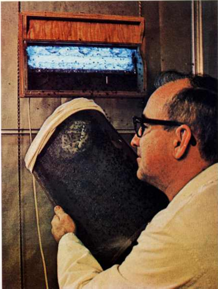
Flies released from cage swarm toward experimental flytrap with ultraviolet lamp as attractant.
