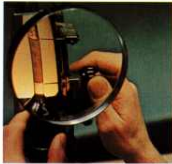
Checking precise butterfat content of milk sample.
