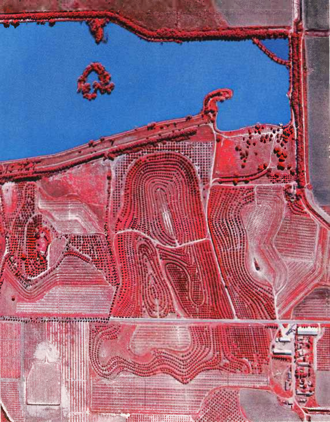
Sensing devices on spacecraft and airplanes are being developed to determine crop condition, detect insect and disease damage, and for other purposes. Here, brown soft scale infestation of citrus trees in Texas is detected at early stage with aerial infrared photo. Infested trees below pond are dark, due to absorption of infrared light by sooty mold from infestation.
