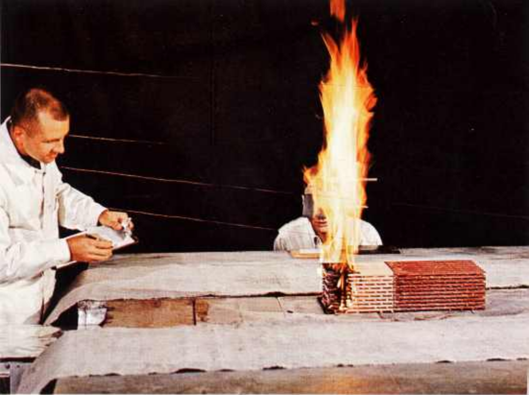
Scientists test effectiveness of fire-retardant chemical for forest fire use. Flames blaze high through untreated wood crib fuel bed, top , then die down, below , on reaching portion treated with chemical.
