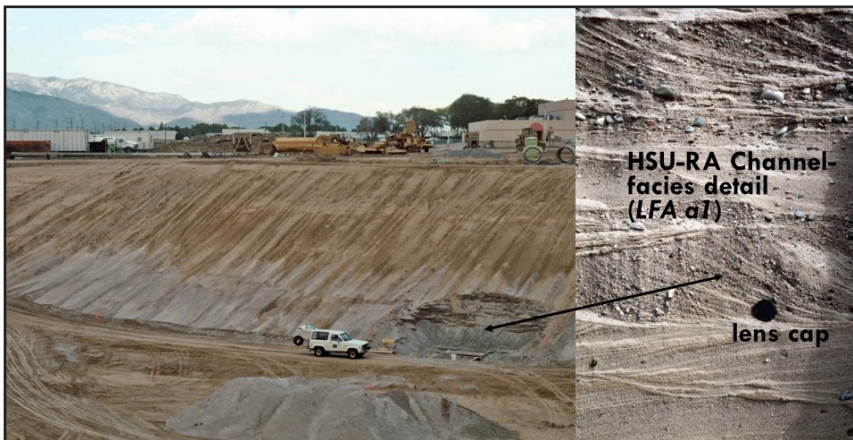
Figure 15. Very high permeability late Pleistocene Rio Grande channel deposits (HSU-RA / LFAa1) exposed in ABCWUA flood basin west of Menaul School and Broadway (1994). Primary component of the river valley's shallow-aquifer system, and a great Managed Aquifer Recharge (MAR) site!
