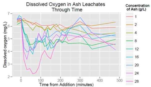
Figure 3: Plot of dissolved oxygen following addition of the fire ash to deionized water. The immediate consumption of oxygen is due to chemicals present in the Juniper ash that readily bind to dissolved oxygen. The chemical oxygen demand will be further studied with Drs. Cerrato and Blake of UNM
