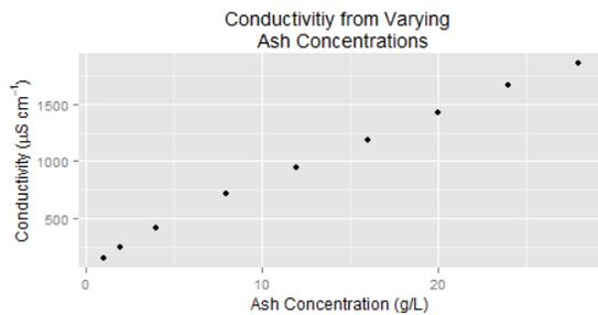
Figure 2: Plot of mean conductivity values following addition of the fire ash to deionized water. The resulting values exceed the conductivity reading from the previous study in the East Fork Jemez River.
