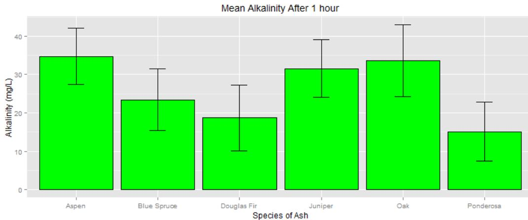
Figure 4: Mean alkalinity of fire ash leachate after one hour. The alkalinity of fire ash can vary between species of tree, though a forest fire will have ash from multiple sources and so will vary from the measured values.
