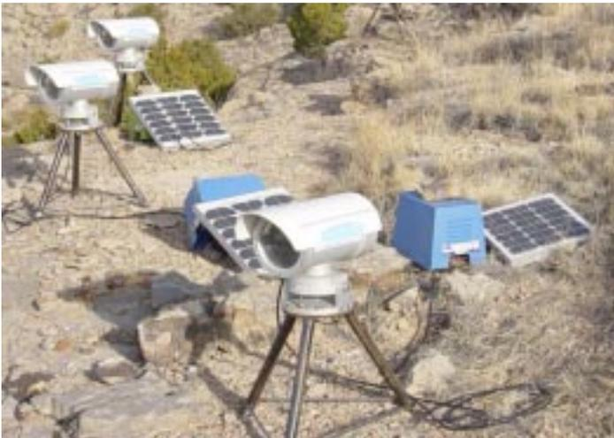
Setup of four instruments during the Scintillometer Intercomparison Study conducted by Kleissl and Hendrickx in the Sevilleta National Wildlife Refuge in Winter 2005.
