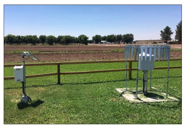
Figure 5. Pluvio rain gauge with wind shield
