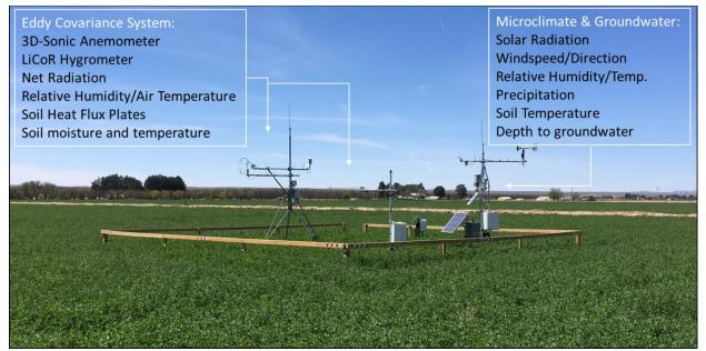
Figure 2. Evapotranspiration (ET) flux tower in 85 acres of alfalfa field
