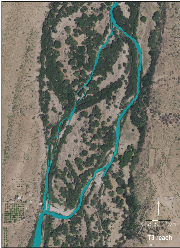
Figure 8. Segment of the upstream study area, near the head of the Cliff-Gila Valley, in 2014. Active floodplain widths in the valley vary from around 400 m to more than 600 m. Much of the floodplain vegetation is distant from water in the river's main channel(s) (blue), often > 100 m distant.
