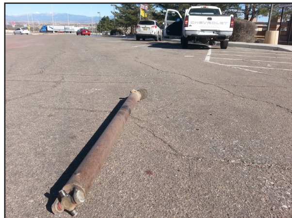
Figure 1. Drive shaft dropped from work truck.
