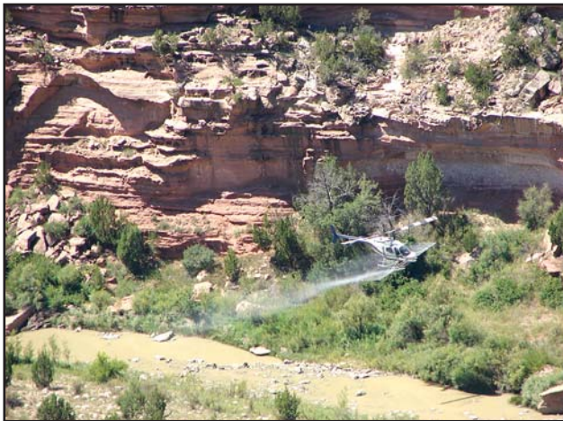
Figure 2. Bell Jet Ranger eradicating salt cedar in Box Canyon of the Canadian River
