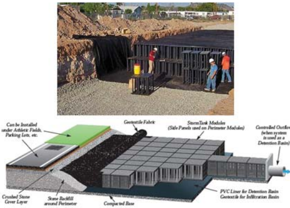
Figure 14. Underground infiltration basins
