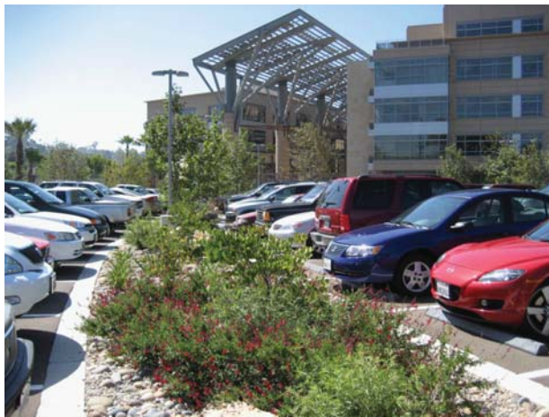
Figure 6. Bio-retention of parking lot runoff in San Diego
