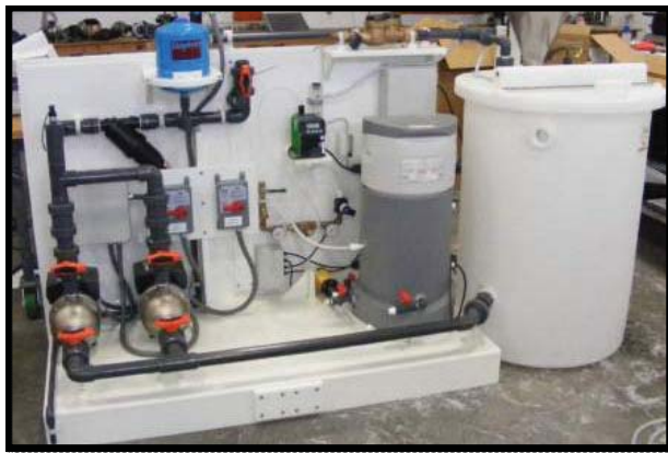
Figure 15. Traditional active mechanical rainwater harvesting components
