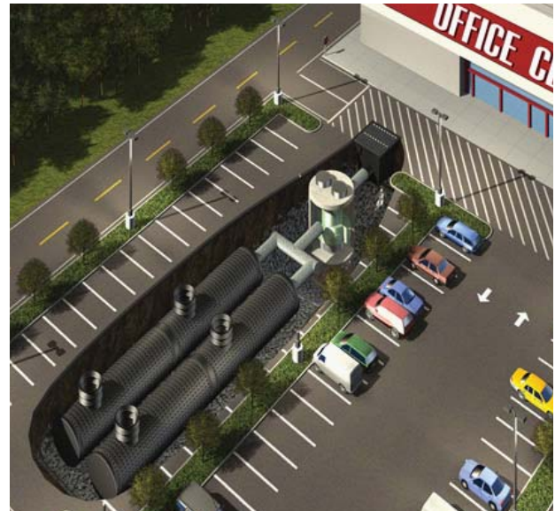
Figure 8. Subsurface infiltration where pretreatment of runoff would be required
