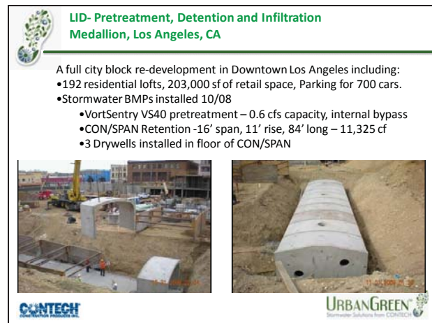
Figure 10. Los Angeles concrete infiltration and drywell system
