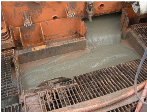
Figure 16. Gray Cement Starting to Emerge from the Annulus
