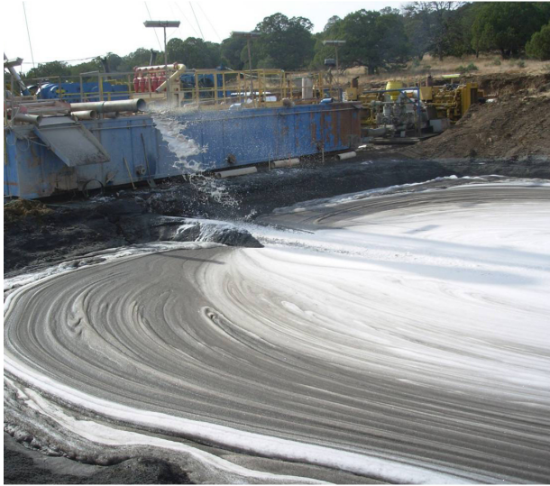
Figure 10. Hubbard Deep Well Initially Drilled on Air/Form
