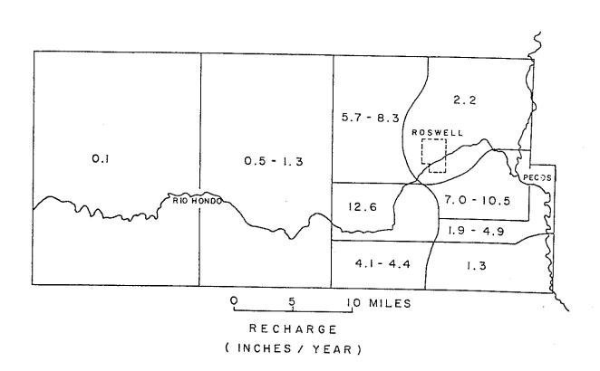
Fig. 7. Calibrated recharge.
