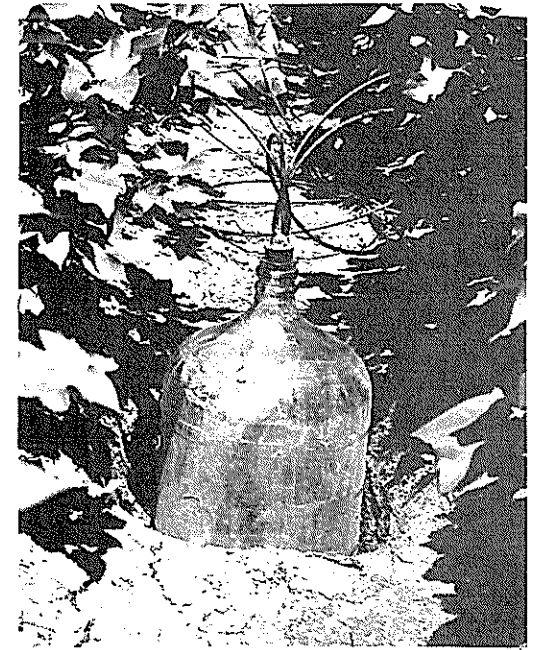
Water that drains below the cotton roots is collected for analysis of salt content.
