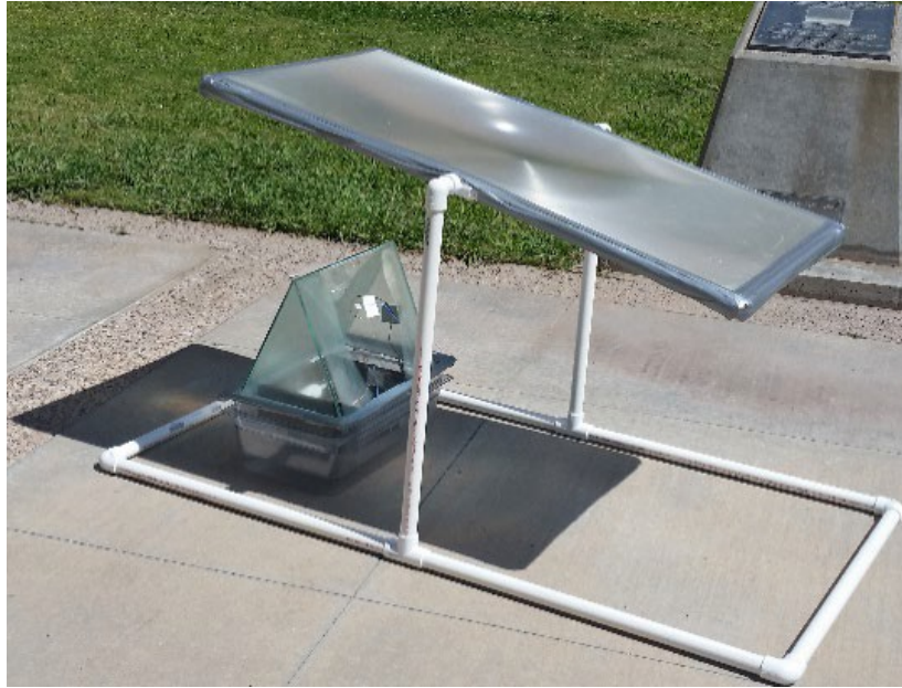
Figure 2-1. Initial design of Solar Still: Test setup with Fresnel lens
