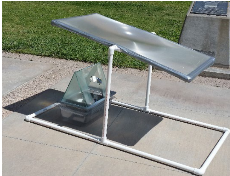
Figure B-2. Solar still test setup with Fresnel lens
