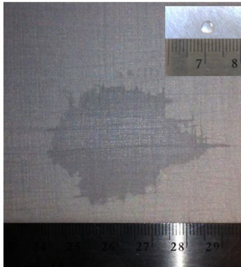
Figure 3-14. A 5 \mu\text{L} water droplet wetting and spreading on a paper towel-like aluminum surface; the inset shows a 5 \mu\text{L} sessile droplet on a polished aluminum surface (polished using 1200 grit paper)
