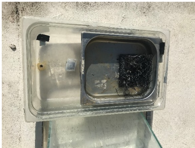
Figure 3-2. Set-up of outdoor solar evaporation with carbon fiber
