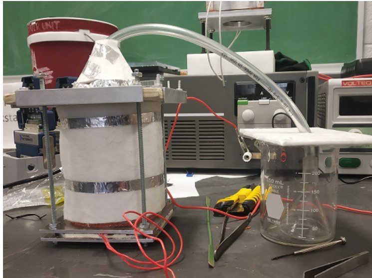
Figure D-1. Test apparatus developed at the laboratory to find corrosion resistance on BiS specimen
