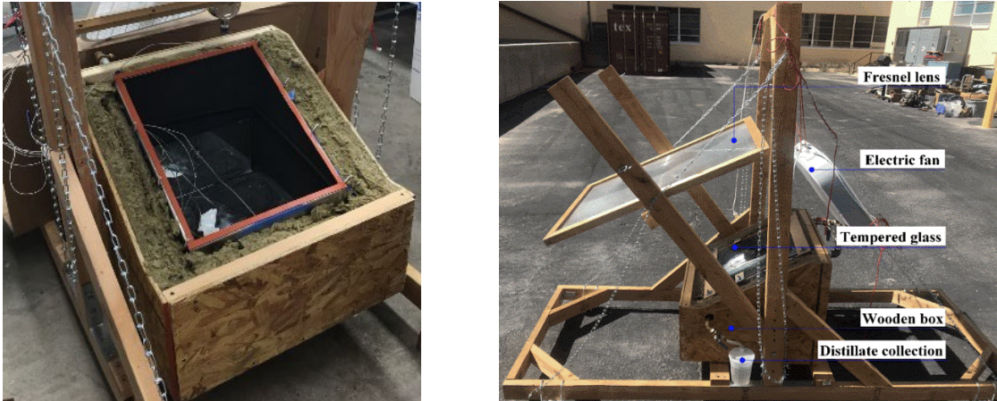
Figure 2-2. Fabricated single-slope still (left), assembled test setup (right)
