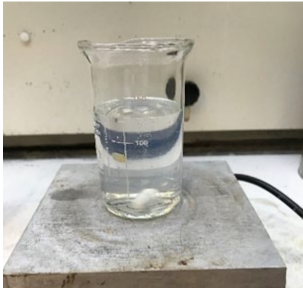
Figure 4-3. Preparation of coating solution
