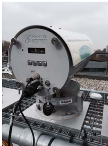
Figure 15. Second generation Kipp & Zonen LAS of New Mexico Tech during calibration in The Netherlands in April 2015.
