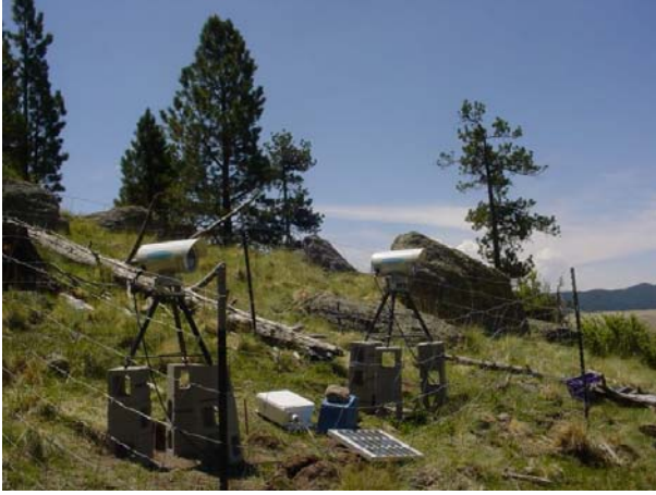
Figure 3. Two LASs (one receiver and one transmitter) during the Scintillometer Intercomparison study in northern NM. The corresponding transmitter and receiver are 2 km away.
