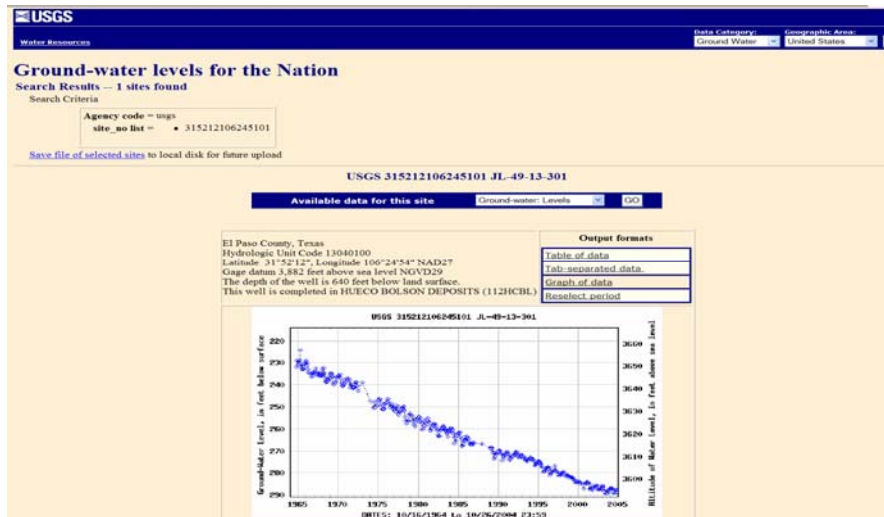
FIGURE 5. USGS Historic Groundwater Level Data for the Texas Well JL-49-13-301 (EPWU MR-3) (USGS 2005)
