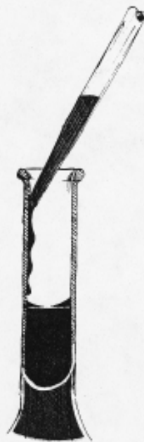
STEP #7 - LINE UP MENISCUS WITH CALIBRATION MARK BY ADDING WATER SLOWLY FROM A PIPET.
