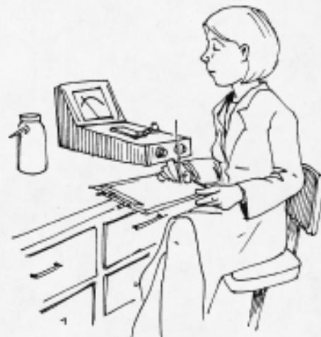
STEP #11 - RECORD THE ABSORBANCE VALUE OBTAINED FROM THE SCALE.
