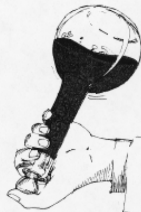
STEP #8 - STOPPER AND INVERT FLASK TO MIX.
