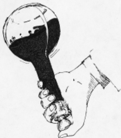
STEP #6 - STOPPER AND INVERT FLASK TO MIX.
