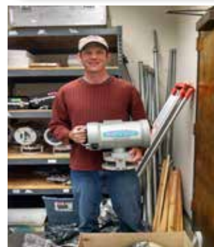
Reid Brown, NM Tech, master's student (Dr. Jan Hendrickx) Test of the new LAS MkII Scintillometer for validation of statewide New Mexico evapotranspiration maps
