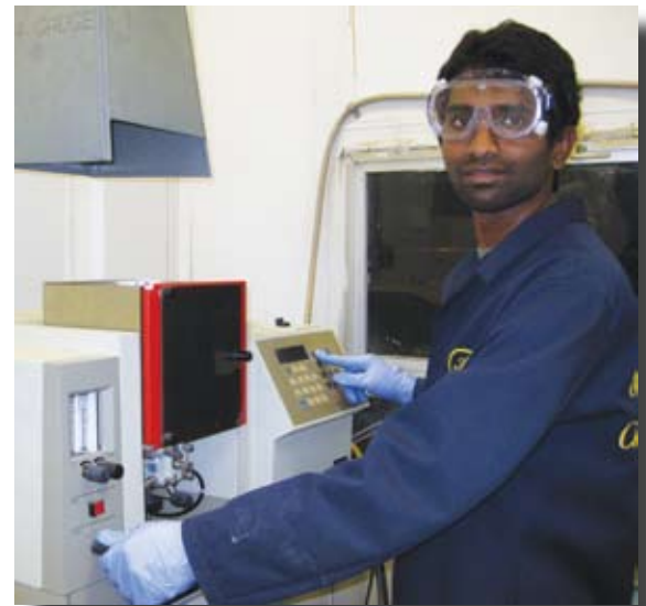
Ranganath Potluri will use this atomic absorption spectroscope in his laboratory to measure the amount of arsenic deposited on the surfaces of the crushed pecan cells.
