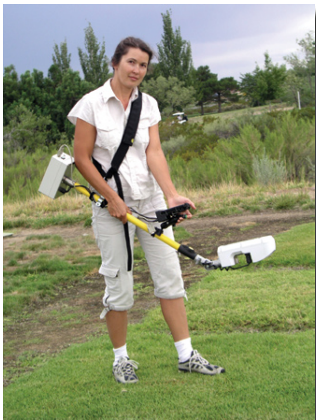
Elena Sevostianova holds a green-seeker, used to monitor changing turfgrass conditions during the growing season.
