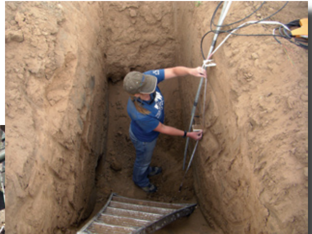
Ciara installs soil water content and temperature probes (top) and plants cottonwood pole cuttings (left).
