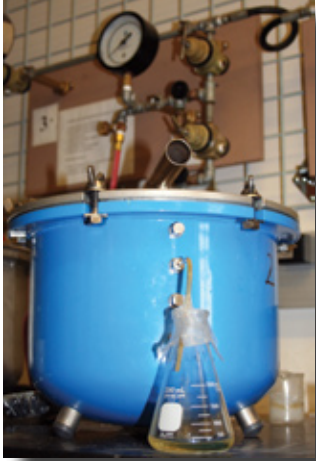
Elena uses an extractor to develop a retention profile for a soil sample.
