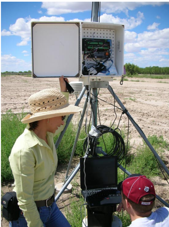
Maritza Macias-Corral and colleague collect ET and climate data at 30-minute intervals using data logger at the Bosque del Apache tower.
