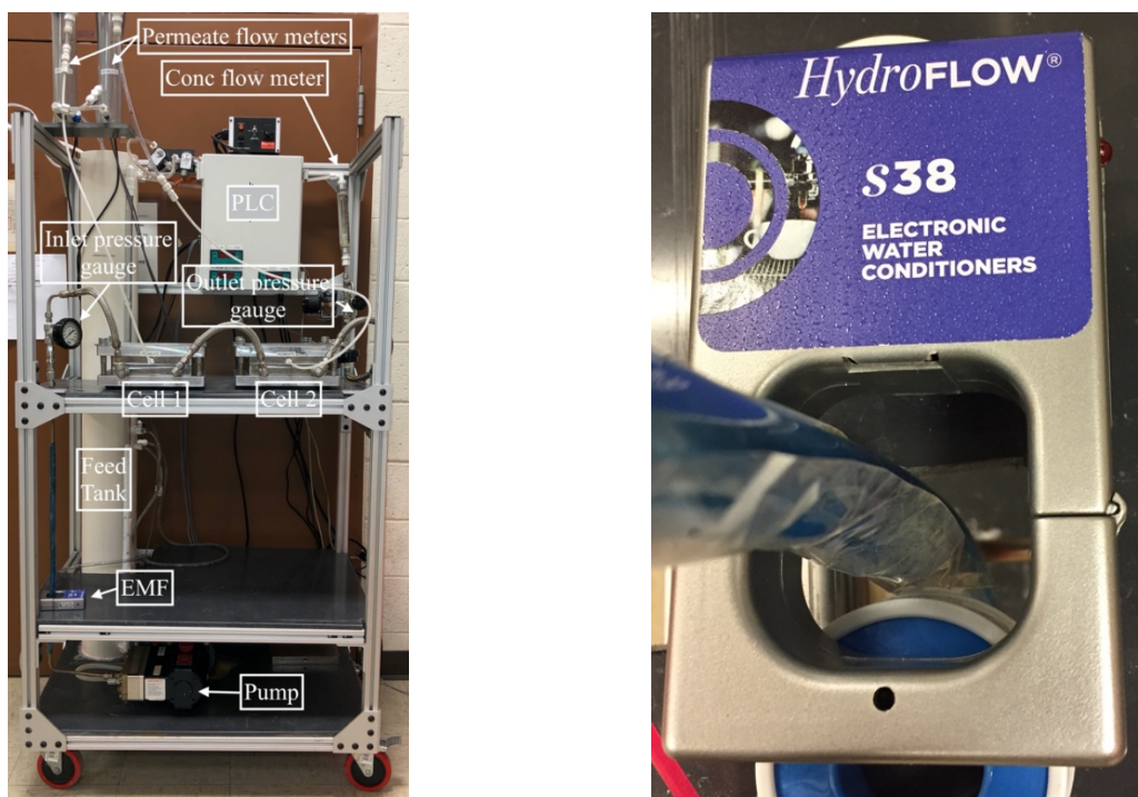
Figure 5. Bench scale RO system (left) and EMF inducer (right)
