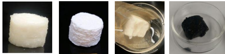
Fig.4: Sample images from poly(AA-co-MBA) and poly(AA-co-MBA)/PPy formation: after curing, washing, soaking in pyrrole solution, and PPy formation (from left to right)
