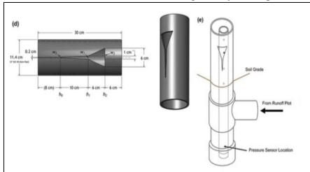
Decagon CTD-10 sensors were utilized to measure water depth within the devices. These sensors use a vented pressure transducer to obtain water level depths from 0 to 10 meters with a resolution of 2 millimeters. Water depth readings are recorded at one minute intervals using Decagon Em50 Data Loggers.
