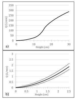
Figure 5: a) Rating curve for UBeTube configuration with correction coefficient of 0.95, and b) Detail of curve at low flows. Dotted lines indicate 2mm resolution of sensors.
