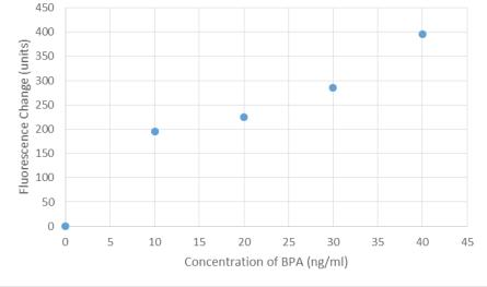
Figure 2 shows the results obtained from the TD700 fluorimeter, which is in this case the most simplistic instrument used. Fluorescence intensity was seen to increase upon addition of increasing concentrations of the aptamer, the opposite of what would be expected. The possibility that BPA itself or the DMSO solvent it was dissolved in were accounting for this increase was explored and ruled out by several experiments. These strange results along with the
