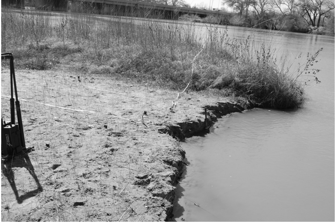
Figure 13 - Northern most edge of the GPR survey site, directly along the Rio Grande. Survey markers, string, the non-conductive tape measure and GPR equipment are visible on the left side of the photograph. Hand probing into the study site after data collection confirmed that depth to water was only several centimeters throughout the study site.
