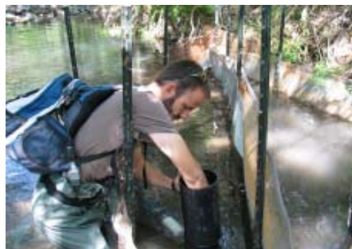
Ryan samples benthic invertebrates, periphyton, and organic matter with a vacuum sampler to be processed in the lab.
